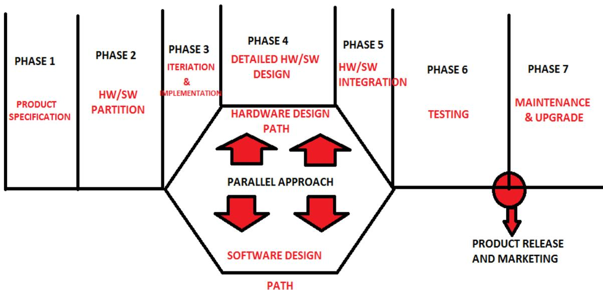
Figure 3 shows Embedded system life cycle and its different phases.
