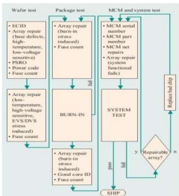
Fig 5 shows eFUSE applications at various test steps
