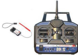
Figure 5. RF transmitter and receiver
