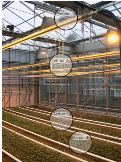
Fig.4. Temperature measurement in the greenhouse
