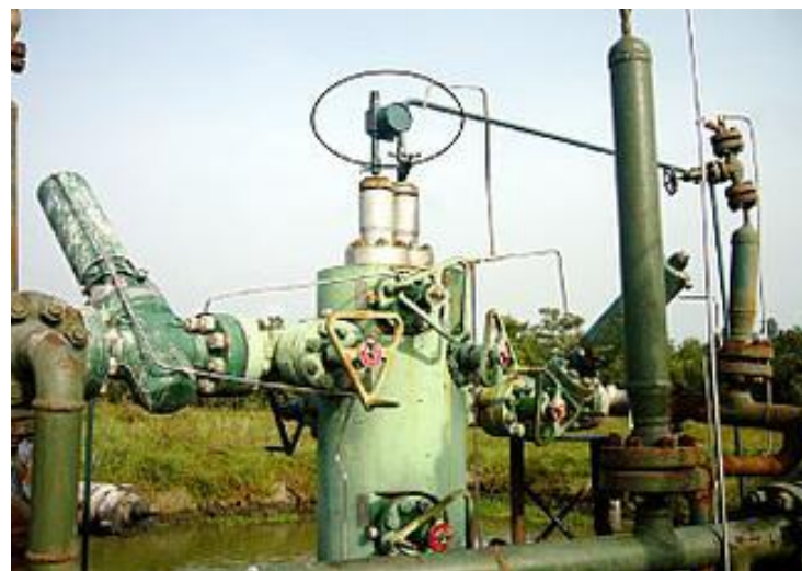
Fig.2. The vMBusX-SP unit is barely noticeable on this well in the Niger Delta, thus providing a feature that helps prevent theft and sabotage [5]
