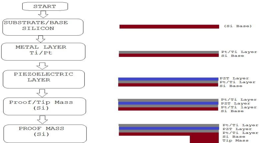
Fig. 2 Fabrication Steps of Piezoelectric Cantilever Beam
