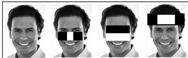
Figure 3: Examples of Haar features. Areas of white and black regions are multiplied by their respective weights and then summed up to get the Haar feature value.
