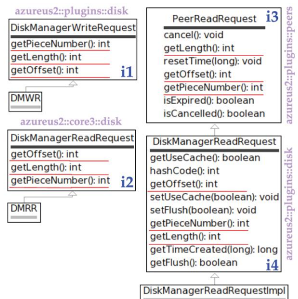
Fig. 1 Example of Interface Similarity. Duplication of read & write request services in four interfaces in Vuze.
