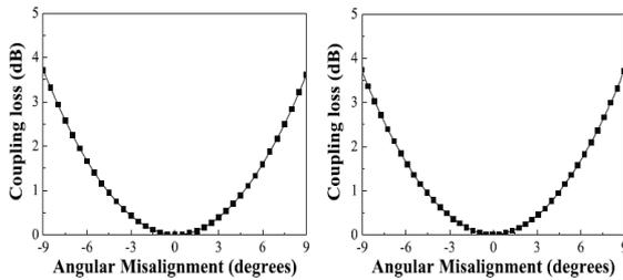
Fig.8 coupling loss against angular misalignment  $\alpha$  (in degrees)
