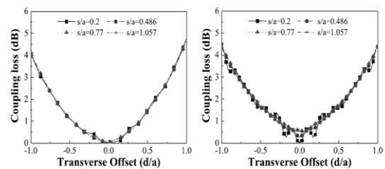
Fig.7 coupling loss against normalized transverse offset
