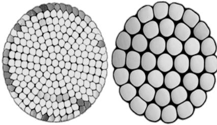
Fig .3 POF (1 mm fibers with 37 and 217 cores)
