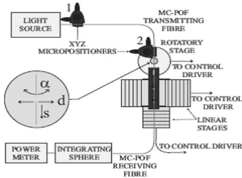
Fig.5 Experimental set-up to measure coupling losses of PF MC-POFs
