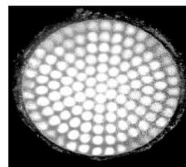
Fig.2 Cross section photograph of the surveyed PF MC-POF
