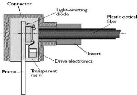
Fig.1 Connector and light source linked with POF
