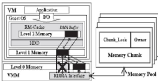
Fig.3. Elastic cache structure and double paging problem
