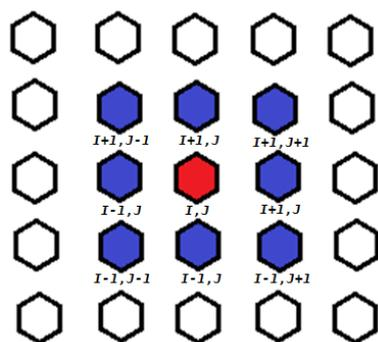
Figure 5. Nine pixel point calculations to generate average and standard deviation. The red pixel and the surrounding eight blue ones are used in calculations of the seven statistical properties of red pixel H-S-V color.
