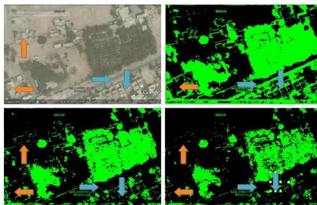
Figure 7. Top left: original image of urban area with manmade vegetation where blue arrows point to roads and houses. Top right: binary image with Phase 1 training where green pixels correspond to vegetation. Bottom left: binary image with Phase 2 training. Bottom right: binary image with Phase 3 training.
