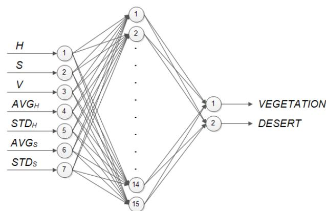
Figure 6. BPNN network used in research with 7 neuron for input layer, 15 neurons for hidden layer, and 2 neurons for output layer.
