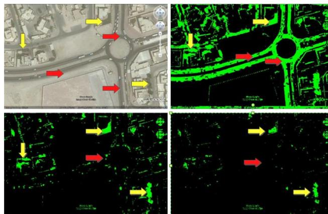
Figure 9. Top left: Original image for urban area with man-made vegetation where blue arrows point to roads and houses. Top right: binary image with Phase 1 training where green pixels correspond to vegetation. Bottom left: binary image with phase 2 training. Bottom right: binary image with Phase 3 training.
