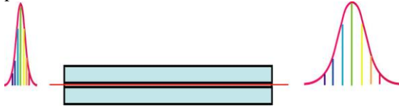
Fig.2. Pulse broadening due to chromatic dispersion
