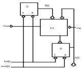
Fig. 2 Accumulator cell
