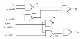
Fig. 5 C17 Benchmark circuit with inputs from accumulator cell output
