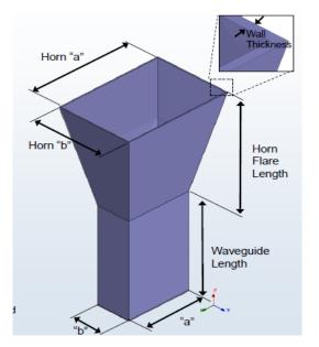
Fig.1 Structure of Proposed Horn Antenna
