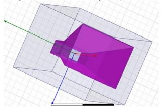
Fig.2 3D view of Pyramidal Horn in HFSS
