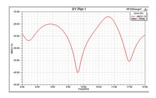
Fig.3 Return loss |s| db over frequency range
