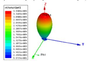
Fig.5 3D Radiation pattern of the antenna in HFSS
