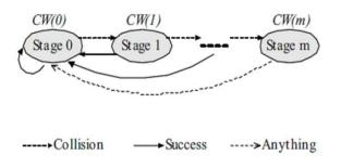
Fig. 1.Operation of 802.11 DCF with BEB Algorithm
