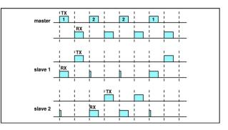
Fig. 6. Master/Slave transmits and receives timings
