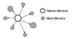
Fig. 1. Piconet master slave Bluetooth architecture
