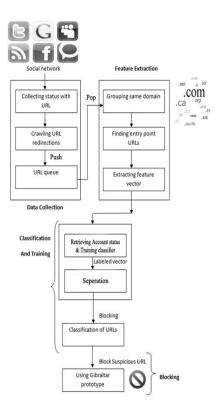
Fig. 2. System Architecture Design
