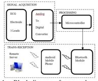
Fig. 1. Block diagram of proposed system
