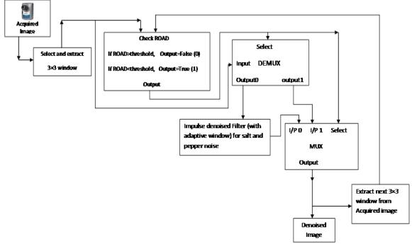
Fig.2: Architecture of Proposed Filter noise.
