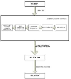
Fig 2 : System design of Hybrid Algorithm
