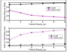
Figure 3 Packet delivery ratio and the end-to-end delay of the HLAR protocol compared to the AODV-ETX protocol as a function of the vehicle density ( $\rho$ ) in [nodes per 2000] m21.
