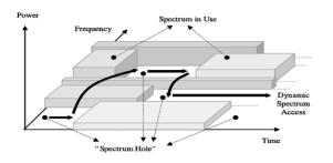
Fig.1 Illustration of spectrum hole
