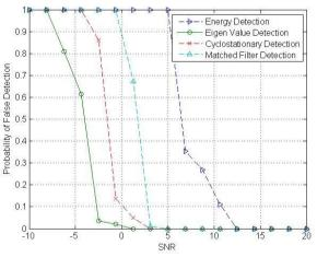
Fig. 5 Probability of false alarm vs SNR
