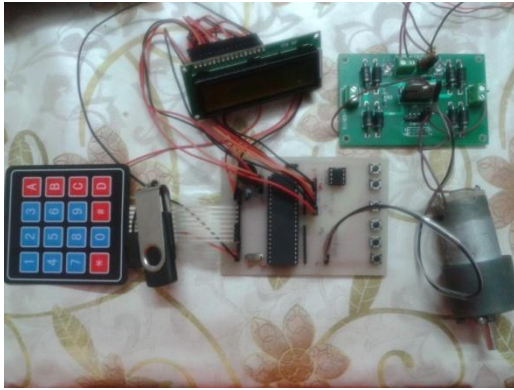
Figure 8 : PCB Testing of PIC MU, LCD, DC Motor
