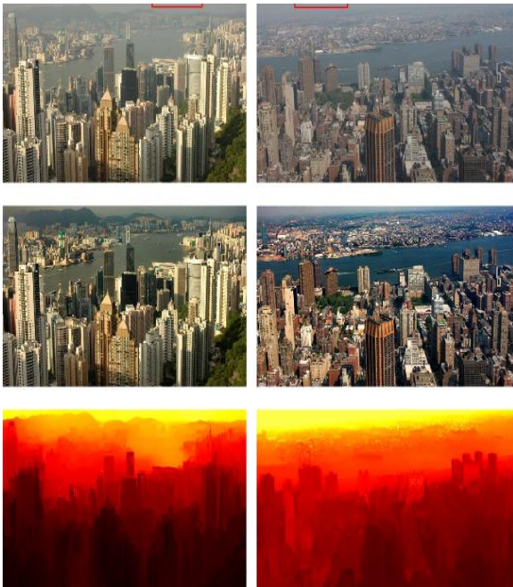
Figure 1: Haze removal results. Top: input haze images. Middle: restored haze-free images. Bottom: depth maps.
