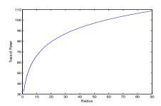
Fig 3. Variation of trace of power with radius
