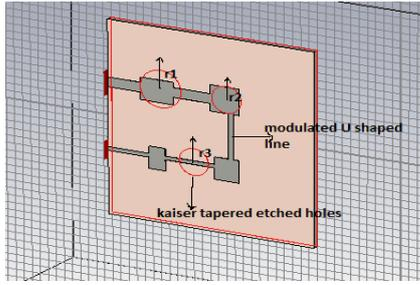
Fig. 3. Non Uniform dual plane Kaiser Tapered EBG Low Pass Filter Structure
