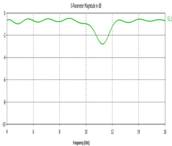
Fig.9. Simulated S21 parameter for Uniform dual plane EBG all pass filter structure with filling factor 0.12
