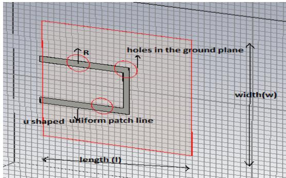
Fig. 1. Uniform dual plane EBG Low Pass Filter Structure
