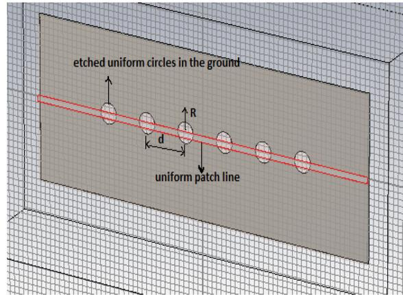
Fig. 2 Uniform dual plane EBG Band stop Filter Structure
