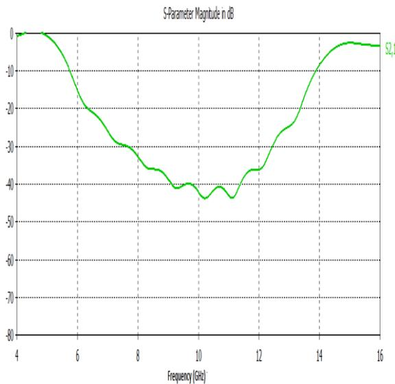
Fig.8. Simulated S21 parameter for non Uniform Kaiser tapered dual plane EBG band stop filter structure
