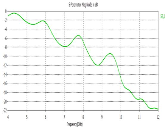
Fig.5. Simulated S21 parameter for Uniform dual plane EBG low pass filter structure
