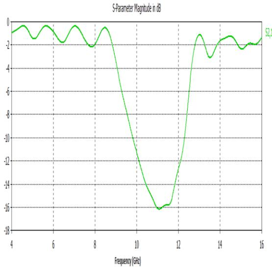
Fig.7. Simulated S21 parameter for Uniform dual plane EBG band stop filter structure
