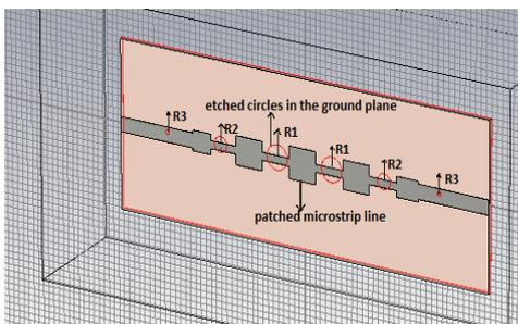
Fig .4. Non Uniform Dual Plane Kaiser Tapered EBG Band stop Filter Structure
