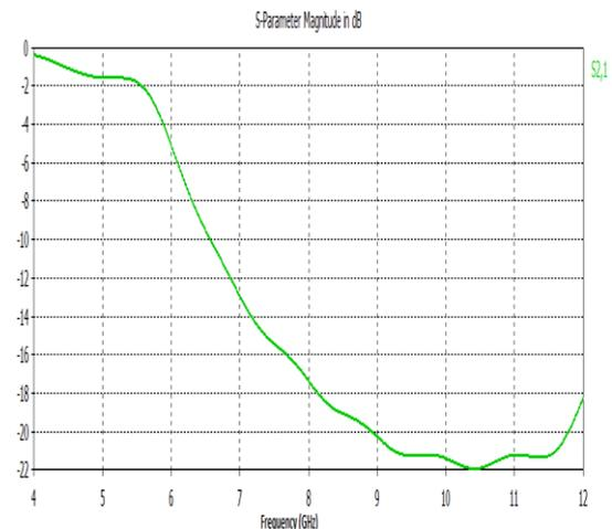
Fig.6. Simulated S21 parameter for non Uniform Kaiser tapered dual plane EBG low pass filter structure
