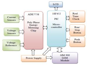
Fig. 3. Block diagram of the Smart meter
