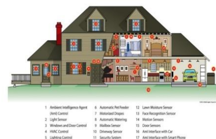
[4]. Fig. depicts various wireless sensors developed for a smarter and safer homes.
