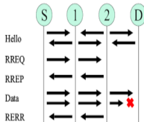
Fig. 1.3: message passing in AODV
