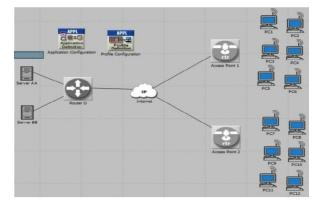
These access points are connected by PPP-DS1 to Router S connected by PPP-DS1 to IP cloud (Internet) connected by PPP-DS1 to Router D connected by PPP-DS1 to two Servers (Server AA, Server BB) which represents two departments.
