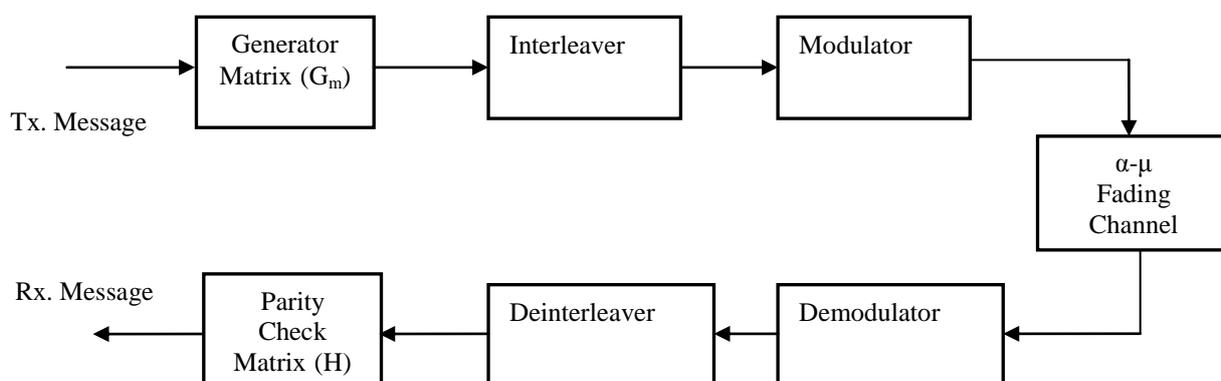
Fig. 2. Block coded communication system considered for simulation
