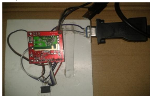
Fig 9: RF Module connected to Server
