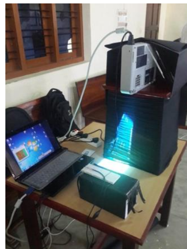
Fig.2. Hardware Setup of Electronic Vein Finder
