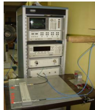
fig. 2.1 VNA Machine for RCS experiment
