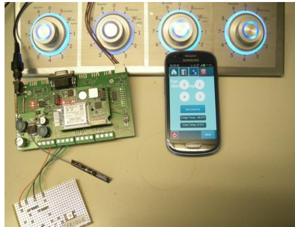
Fig 1: Android mobile is showing stove top status
