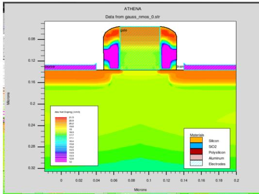
Figure: 1 Athena structure of 45nm NMOS
