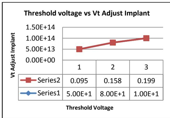
Figure: 5 Variation of threshold voltage at different  $V_t$  adjust implantation
