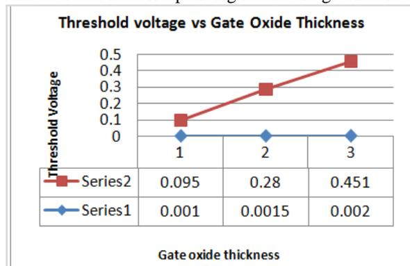
Figure: 4 Threshold voltages at different gate oxide thickness.
