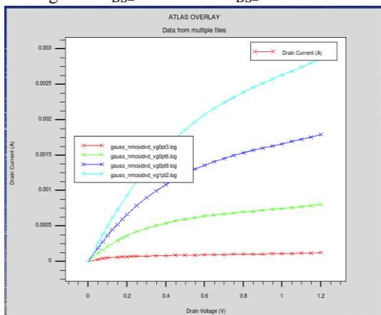
Figure: 3 ID-VDS curve at various gate voltages
