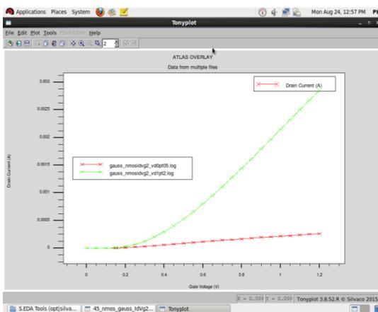
Figure: 2 ID-VGS curve at different drain voltages
