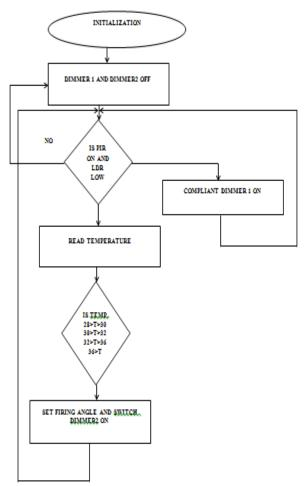
Fig. 4. Software description flowchart for lighting
