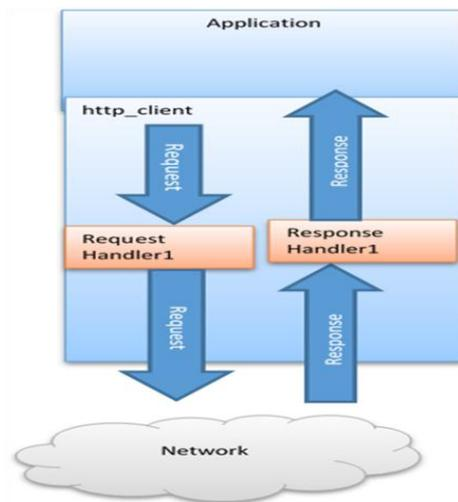
Fig6.1:Structure of request & Response message on Server
