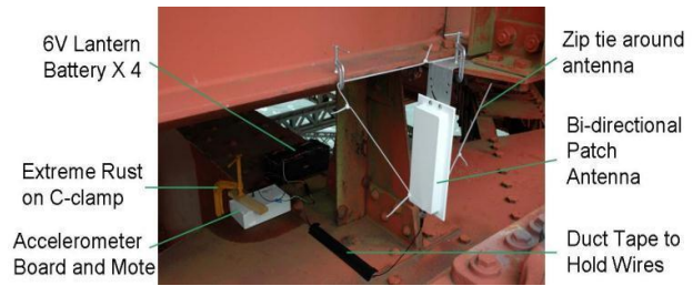
Fig 4: Placement of actual system for SHM in GGB
