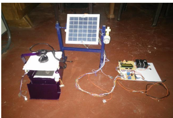
Fig 5: Hardware setup for Coin based mobile charger using solar panel
