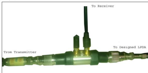
Fig.7. Connector setting to measure reflected power
