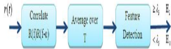
Figure 4 Block diagram of cyclostationary detection [7]
