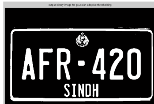
Fig. 4. Output binary image for Gaussian adaptive thresholding
