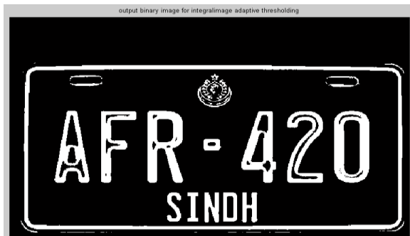
Fig. 5. Output binary image for Integral image
