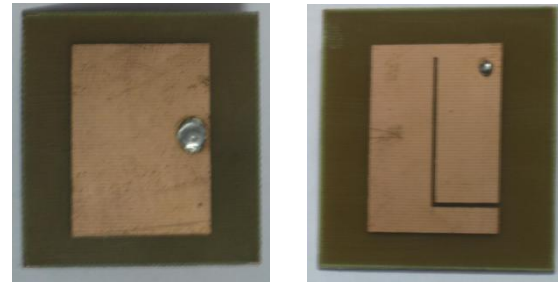
Fig.7 Hardware Design of (a) Rectangular patch antenna (b) L-shape slotted patch antenna
