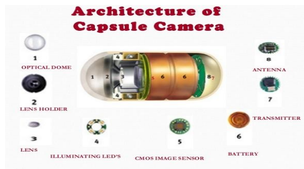
Fig 3.4 Components of Capsule Camera
