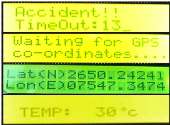
Fig10 displays gps co-ordinates after accident detection and temperature
