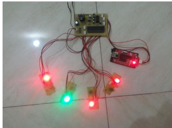
Fig 7. Traffic Control Unit Displaying Traffic Signals
