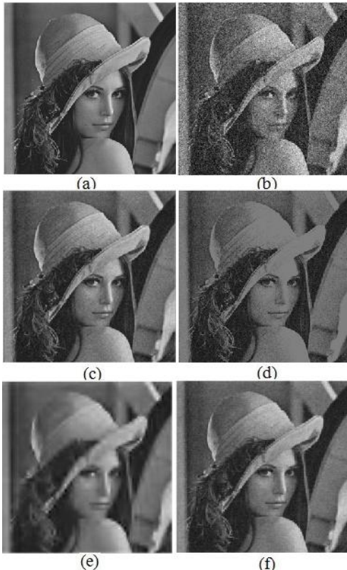
a)Original image, b) Noisy image, c) Average filter, d) VisuShrink, e) SureShrink, f)Adaptive thresholding
