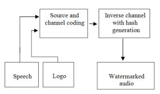
In source and channel coding process contain inputs audio and image. In source coding SPIHT algorithm is used for image compression. In channel coding DCT techniques are used for maximum to minimum pixel after encoding process this data is given to input of inverse channel coding with has generation Hash information which was derived from the image blocks in are now extracted from Extraction process: the speech frames finally watermarked audio is generated
