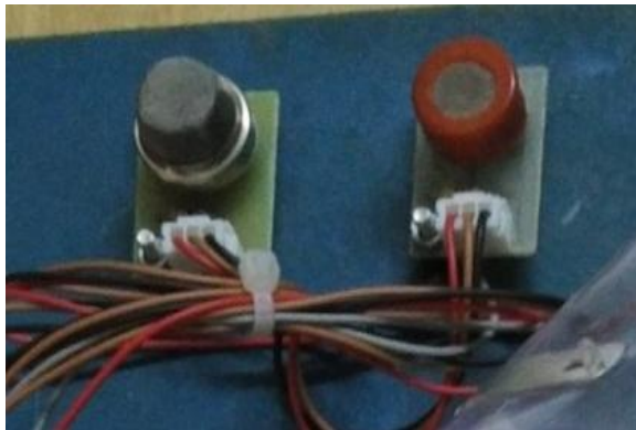
Fig. 2. CO and CO 2 sensors
