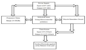
Figure 2: Functional Block Diagram of Rehabilitation Muscle Stimulator
