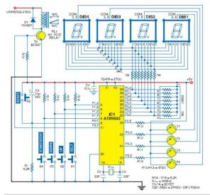
Figure 3:Circuit Diagram of Industrial Timer
