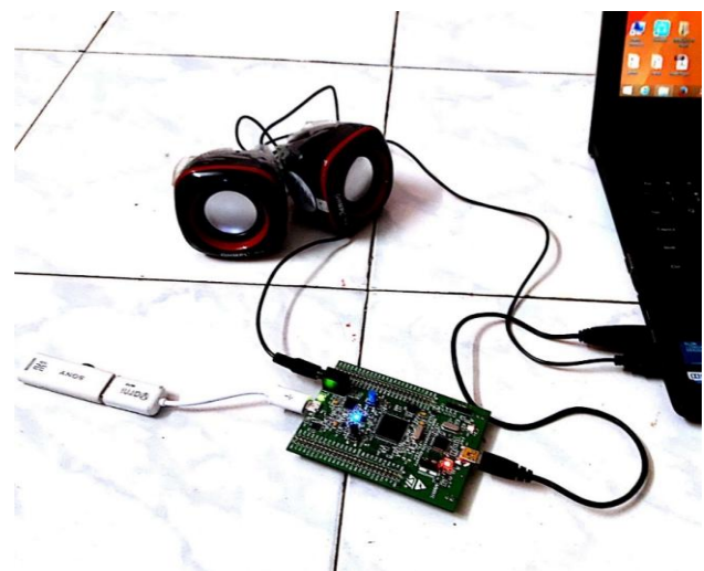
Fig. 9. Playback mode (Blue led blinking)
